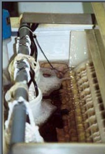
A small barrel of parts rotates in the silver bath. Silver is the most conductive metal, however, it requires a copper or nickel undercoat.
